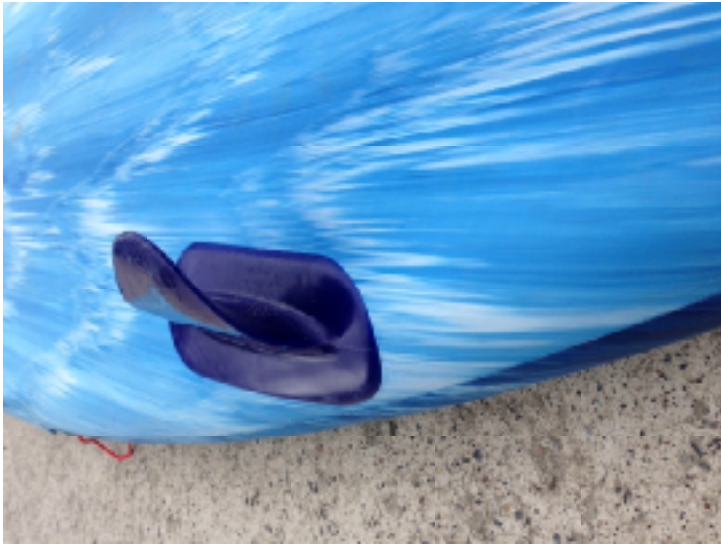
1. This picture shows a bent fin.
