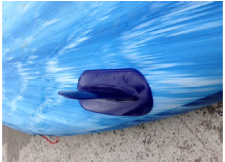
4. Allow to cool either naturally or by pouring cold water over the fin. You should find your fin is now straight.
