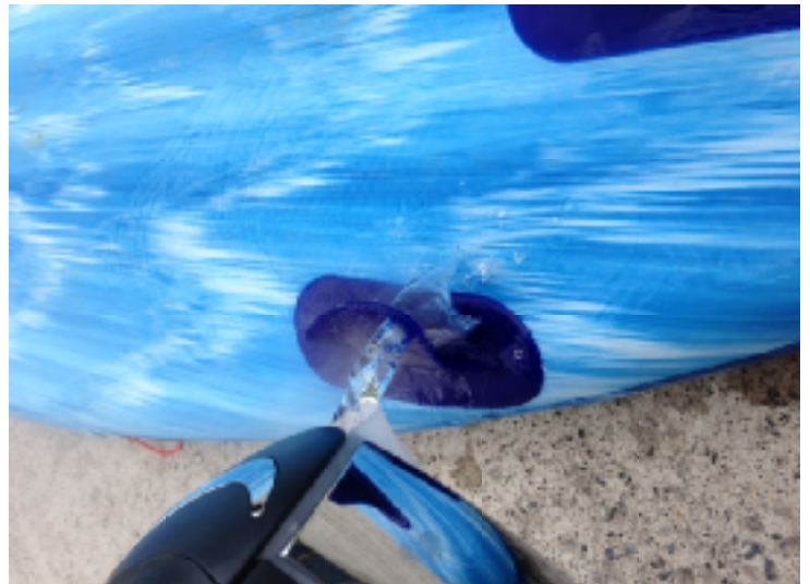
2. Pour hot water from the kettle on to the fin to make the fin flexible.
