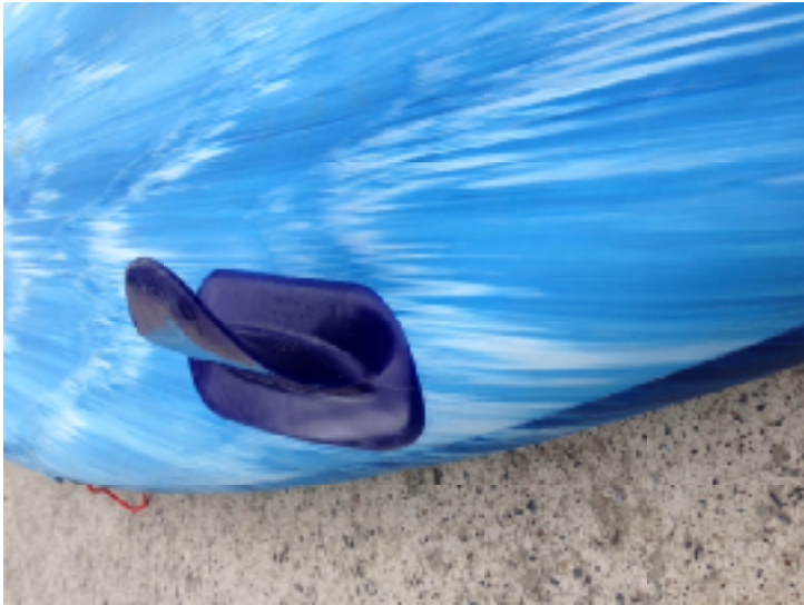
1. This picture shows a bent fin.
